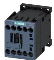
power contactor, AC-3e/AC-3, 9 A, 4 kW / 400 V, 3-pole, 400 V AC, 50/60 Hz, auxiliary contacts: 1 NC, screw terminal, size: S00
