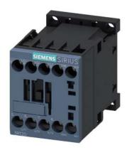
power contactor, AC-3e/AC-3, 7 A, 3 kW / 400 V, 3-pole, 24 V DC,  $0.85-1.85^{*}$  Us, auxiliary contacts: 1 NC, screw terminal, size: S00, not expandable with auxiliary switch
