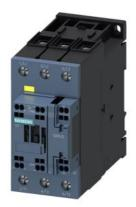
power contactor, AC-3e/AC-3, 80 A, 37 kW / 400 V, 3-pole, 21-33 V AC/DC, 50/60 Hz, with integrated varistor, auxiliary contacts: 1 NC, main circuit: screw terminal, control and auxiliary circuit: spring-loaded terminal, size: S2, F-PLC-IN
