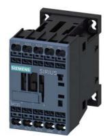
power contactor, AC-3e/AC-3, 12 A, 5.5 kW / 400 V, 3-pole, 230 V AC, 50/60 Hz, auxiliary contacts: 1 NC, spring-loaded terminal, size: S00, upright mounting position
