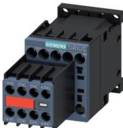
power contactor, AC-3e/AC-3, 7 A, 3 kW / 400 V, 3-pole, 230 V AC, 50/60 Hz, auxiliary contacts: 2 NO + 2 NC, screw terminal, size: S00, captive auxiliary switch
