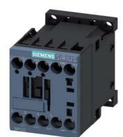
power contactor, AC-3e/AC-3, 7 A, 3 kW / 400 V, 3-pole, 24 V DC, auxiliary contacts: 1 NO, screw terminal, size: S00, communication-capable
