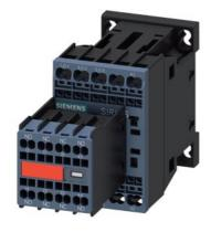
power contactor, AC-3e/AC-3, 9 A, 4 kW / 400 V, 3-pole, 24 V DC, with integrated diode, auxiliary contacts: 2 NO + 2 NC, spring-loaded terminal, size: S00, captive auxiliary switch
