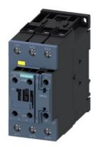
power contactor, AC-3e/AC-3, 65 A, 30 kW / 400 V, 3-pole, 21-33 V AC/DC, 50/60 Hz, with integrated varistor, auxiliary contacts: 1 NC, screw terminal, size: S2, F-PLC-IN
