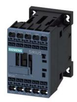
power contactor, AC-3e/AC-3, 9 A, 4 kW / 400 V, 3-pole, 24 V DC, with integrated diode, auxiliary contacts: 1 NO, spring-loaded terminal, size: S00  $\,$
