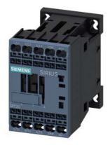
power contactor, AC-3e/AC-3, 12 A, 5.5 kW / 400 V, 3-pole, 24 V DC, auxiliary contacts: 1 NC, spring-loaded terminal, size: S00  $\,$
