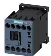
power contactor, AC-3e/AC-3, 12 A, 5.5 kW / 400 V, 3-pole, 110 V AC, 50 Hz / 120 V, 60 Hz, auxiliary contacts: 1 NC, screw terminal, size: S00
