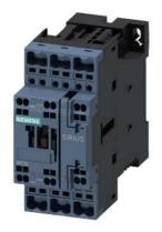
power contactor, AC-3e/AC-3, 12 A, 5.5 kW / 400 V, 3-pole, 200-280 V AC/DC, 50/60 Hz, with integrated varistor, auxiliary contacts: 1 NO + 1 NC, spring-loaded terminal, size: S0
