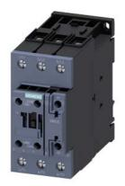
power contactor, AC-3e/AC-3, 65 A, 30 kW / 400 V, 3-pole, 230 V AC, 50/60 Hz, auxiliary contacts: 1 NO + 1 NC, screw terminal, size: S2  $\,$
