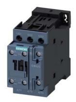
power contactor, AC-3e/AC-3, 9 A, 4 kW / 400 V, 3-pole, 95-130 V AC/DC, 50/60 Hz, with integrated varistor, auxiliary contacts: 1 NO + 1 NC, screw terminal, size: S0
