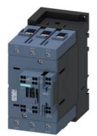
power contactor, AC-3e/AC-3, 95 A, 45 kW / 400 V, 3-pole, 230 V AC, 50/60 Hz, auxiliary contacts: 1 NO + 1 NC, main circuit: screw terminal, control and auxiliary circuit: spring-loaded terminal, size: S3
