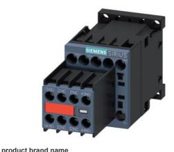
power contactor, AC-3e/AC-3, 7 A, 3 kW / 400 V, 3-pole, 24 V DC, with integrated diode, auxiliary contacts: 2 NO + 2 NC, screw terminal, size: S00, captive auxiliary switch
