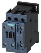
power contactor, AC-3e/AC-3, 9 A, 4 kW / 400 V, 3-pole, 400 V AC, 50 Hz / 400-440 V, 60 Hz, auxiliary contacts: 1 NO + 1 NC, screw terminal, size: S0
