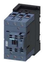
power contactor, AC-3e/AC-3, 95 A, 45 kW / 400 V, 3-pole, 83-155 V AC/DC, 50/60 Hz, with integrated varistor, auxiliary contacts: 1 NO + 1 NC, main circuit: screw terminal, control and auxiliary circuit: spring-loaded terminal, size: S3
