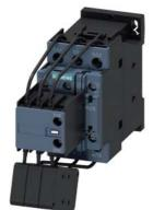
capacitor contactor, AC-6b 25 kVAr, / 400 V, 3-pole, 110 V AC, 50 Hz / 120 V, 60 Hz, auxiliary contacts: 1 NO + 2 NC, screw terminal, size: S0
