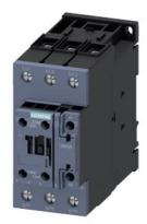
power contactor, AC-3e/AC-3, 65 A, 30 kW / 400 V, 3-pole, 83-155 V AC/DC, 50/60 Hz, with integrated varistor, auxiliary contacts: 1 NO + 1 NC, screw terminal, size: S2
