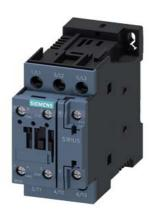
power contactor, AC-3e/AC-3, 9 A, 4 kW / 400 V, 3-pole, 24 V DC, auxiliary contacts: 1 NO + 1 NC, screw terminal, size: S0, communication-capable
