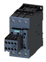
power contactor, AC-3e/AC-3, 65 A, 30 kW / 400 V, 3-pole, 24 V DC, 0.8-1.2\* Us, with integrated varistor, auxiliary contacts: 2 NO + 2 NC, screw terminal, size: S2, suitable for PLC outputs
