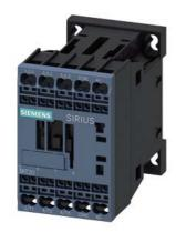
power contactor, AC-3e/AC-3, 7 A, 3 kW / 400 V, 3-pole, 110 V AC, 50/60 Hz, auxiliary contacts: 1 NC, spring-loaded terminal, size: S00  $\,$
