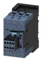
power contactor, AC-3e/AC-3, 95 A, 45 kW / 400 V, 3-pole, 20-33 V AC/DC, 50/60 Hz, with integrated varistor, auxiliary contacts: 2 NO + 2 NC, screw terminal, size: S3, removable auxiliary switch
