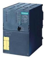
\*\*\*Spare part\*\*\* SIMATIC S7-300, CPU 317F-2DP, Central processing unit with 1024 KB work memory, 1st interface MPI/DP 12 Mbit/s, 2nd interface DP master/slave Micro Memory Card required Can be used with software package S7 Distributed Safety V5.2 SP1 or higher
