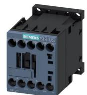
power contactor, AC-3e/AC-3, 12 A, 5.5 kW / 400 V, 3-pole, 400 V AC, 50 Hz / 400-440 V, 60 Hz, auxiliary contacts: 1 NC, screw terminal, size: S00
