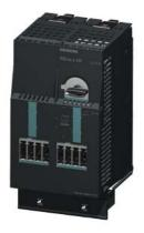
RS1E-X for ET200S High Feature reversing starter Setting range 2.4...8 A Mechanical switching Electronic protection AC-3, up to 3 kW / 400 V expandable for Brake control module 2DI module 2DI module Motor starter ES Circuit breaker signaling parameterizable DPV 1-capable PROFIENERGY-capable to PN
