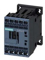
power contactor, AC-3e/AC-3, 12 A, 5.5 kW / 400 V, 3-pole, 110 V AC, 50 Hz / 120 V, 60 Hz, auxiliary contacts: 1 NO, spring-loaded terminal, size: S00
