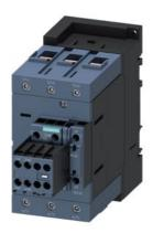
power contactor, AC-3e/AC-3, 95 A, 45 kW / 400 V, 3-pole, 24 V AC, 50 Hz, auxiliary contacts: 2 NO + 2 NC, screw terminal, size: S3, removable auxiliary switch
