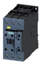
power contactor, AC-3e/AC-3, 80 A, 37 kW / 400 V, 3-pole, 175-280 V AC/DC, 50/60 Hz, with integrated varistor, auxiliary contacts: 1 NC, screw terminal, size: S2, F-PLC-IN
