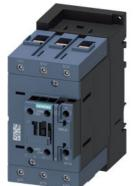
power contactor, AC-3e/AC-3, 95 A, 45 kW / 400 V, 3-pole, 230 V AC, 50/60 Hz, auxiliary contacts: 1 NO + 1 NC, screw terminal, size: S3  $\,$
