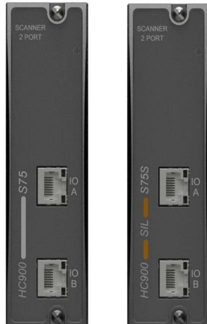
**Process Scanner (left) Safety Scanner (right)**
