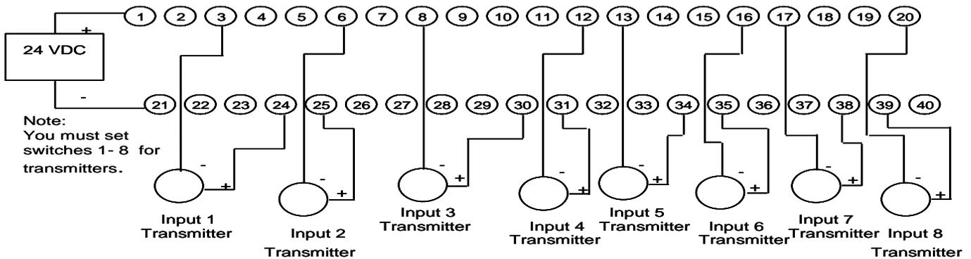
**Remote Terminal Panel for Analog Input Modules (900RTA-xxxx) (cont'd)**
