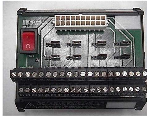
Jumpers on the Remote Terminal Panel may be positioned to accommodate the above input and output modules. A switch on the module is used to disconnect field power from I/O modules to facilitate maintenance of the module under instrument power.
