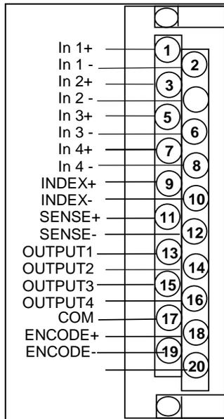
Note: For Quadrature input Differential mode, connect wires using reverse polarity (+ to -) on Input 1, Input 2 and Index.
