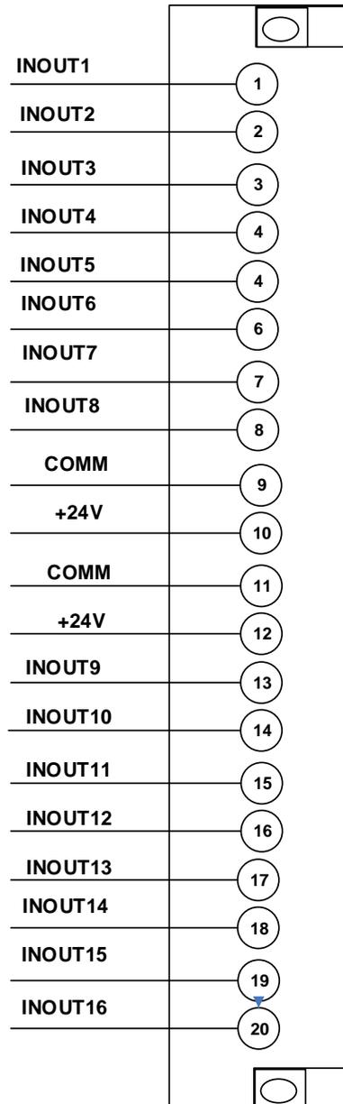
Universal IO channel can be soft configured as AI, AO, DI or DO. Details of each IO type are listed in tables below.
