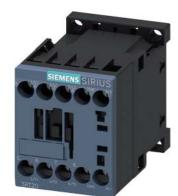
power contactor, AC-3e/AC-3, 7 A, 3 kW / 400 V, 3-pole, 110 V DC, auxiliary contacts: 1 NC, screw terminal, size: S00
