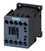
Power contactor, AC-3 7 A, 3 kW / 400 V 1 NC, 24 V DC 3-pole, Size S00 screw terminal
