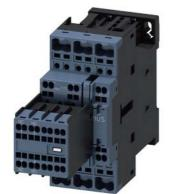
power contactor, AC-3e/AC-3, 9 A, 4 kW / 400 V, 3-pole, 230 V AC, 50 Hz, auxiliary contacts: 2 NO + 2 NC, spring-loaded terminal, size: S0, removable auxiliary switch
