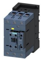
power contactor, AC-3e/AC-3, 110 A, 55 kW / 400 V, 3-pole, 21-33 V AC/DC, 50/60 Hz, with integrated varistor, auxiliary contacts: 1 NC, screw terminal, size: S3, F-PLC-IN
