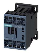
power contactor, AC-3e/AC-3, 9 A, 4 kW / 400 V, 3-pole, 24 V DC, 0.7-1.25 $^{\circ}$  Us, with integrated suppressor diode, auxiliary contacts: 1 NC, spring-loaded terminal, size: S00, suitable for PLC outputs, not expandable with auxiliary switch
