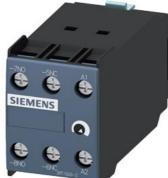
solid-state time-delayed front-side auxiliary switch Time range 5...100 s, 100 ... 127 V AC / DC, 1 NO contact, 1 NC contact OFF delay, without control signal for 3RT1
