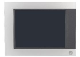
Automation Panel 15.0" XGA TFT -  $1024 \times 768$  pixels (4:3) - Single-touch (analog resistive) - Control cabinet installation - Landscape format - Front USB - For PPC900/PPC2100/PPC3100/PPC2200 - For link modules - Compatible with 5PP520.1505-00, 5AP920.1505-01, 5PC720.1505-xx, 5PC820.1505-00
