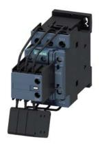
capacitor contactor, AC-6b 20 kVAr, / 400 V, 3-pole, 110 V AC, 50 Hz / 120 V, 60 Hz, auxiliary contacts: 1 NO + 2 NC, screw terminal, size: S0
