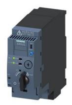
SIRIUS Compact load feeder DOL starter 690 V 24 V AC/DC 50...60 Hz 0.1...0.4 A IP20 Connection main circuit: plug-in, without terminals Connection auxiliary circuit: plug-in, without terminals
