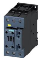
power contactor, AC-3e/AC-3, 65 A, 30 kW / 400 V, 3-pole, 83-150 V AC/DC, 50/60 Hz, with integrated varistor, auxiliary contacts: 1 NC, screw terminal, size: S2, F-PLC-IN
