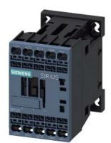
power contactor, AC-3e/AC-3, 7 A, 3 kW / 400 V, 3-pole, 24 V DC, 0.7-1.25\* Us, with integrated suppressor diode, auxiliary contacts: 1 NO, spring-loaded terminal, size: S00, suitable for PLC outputs, not expandable with auxiliary switch
