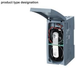
Battery housing for RTU3000C range with autonomous power supply Battery enclosure for holding two mono cells; Suitable for SIMATIC RTU3000C family; Batteries must be purchased separately and are not in the scope of delivery. Observe note regarding battery type in the Equipment Manual!
