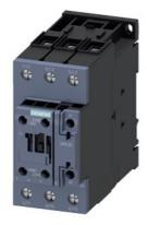
power contactor, AC-3e/AC-3, 80 A, 37 kW / 400 V, 3-pole, 175-280 V AC/DC, 50/60 Hz, with integrated varistor, auxiliary contacts: 1 NO + 1 NC, screw terminal, size: S2
