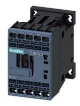
power contactor, AC-3e/AC-3, 12 A, 5.5 kW / 400 V, 3-pole, 24 V DC, 0.7-1.25\* Us, auxiliary contacts: 1 NO, spring-loaded terminal, size: S00, suitable for PLC outputs, not expandable with auxiliary switch
