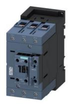
power contactor, AC-3e/AC-3, 110 A, 55 kW / 400 V, 3-pole, 110 V AC, 50 Hz, auxiliary contacts: 1 NO + 1 NC, screw terminal, size: S3  $\,$
