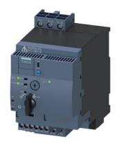
SIRIUS Compact load feeder Reversing starter 690 V 110...240 V AC/DC 50...60 Hz 0.32...1.25 A IP20 Connection main circuit: Screw terminal Connection control circuit: screw terminal
