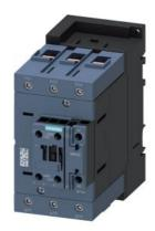
power contactor, AC-3e/AC-3, 110 A, 55 kW / 400 V, 3-pole, 110 V AC, 50 Hz / 120 V, 60 Hz, auxiliary contacts: 1 NO + 1 NC, screw terminal, size: S3  $\,$
