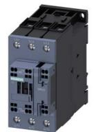
power contactor, AC-3e/AC-3, 65 A, 30 kW / 400 V, 3-pole, 110 V AC, 50/60 Hz, auxiliary contacts: 1 NO + 1 NC, main circuit: screw terminal, control and auxiliary circuit: spring-loaded terminal, size: S2
